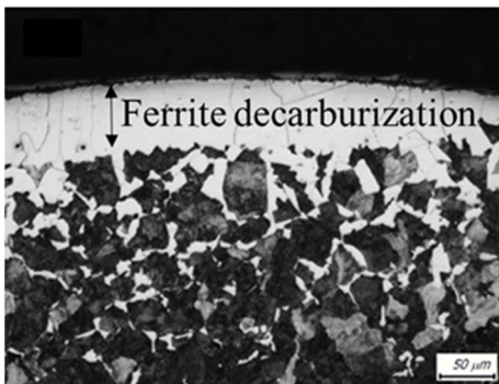
Fig.1. Ferrite decarburization in OM morphology
